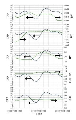
**Fig.5.** Curves of IRP and tuyere practices varied over time during normal operation.
